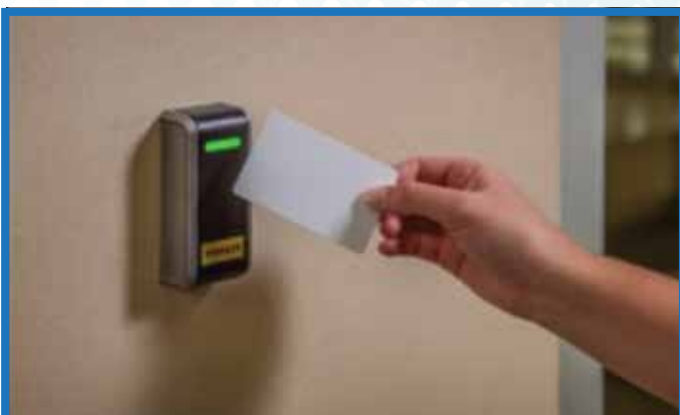
Access Control System
